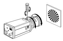
The following describes how to adjust the Back Focus when using a Zoom lens.
